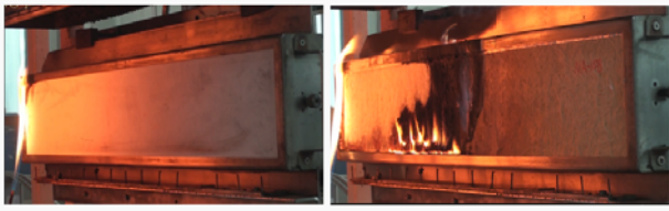
Figure 2: Some of test specimens before the test and after the flame-spread test
