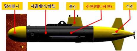
Figure 1: Structure of a typical UUV
