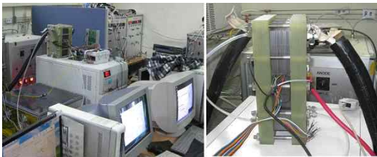
Figure 5: Stack activation Test
