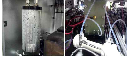
Figure 14: Discharged water sampling with the fuel recirculation flow
