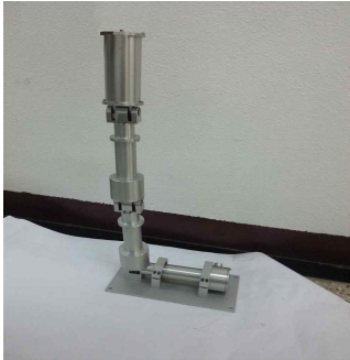
Figure 5: Developed 4-axis waterproof robot arm
