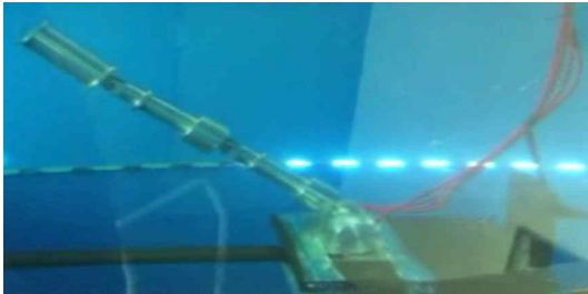
Figure 6: Water proof test of 1st Actuator
