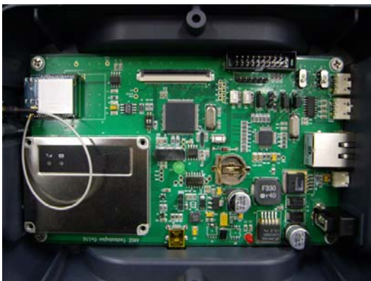
Figure 9 : The Board of the Repeater
