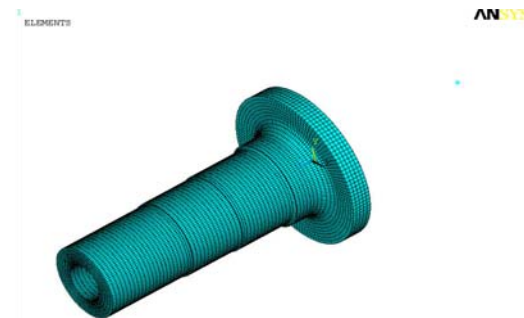
Figure 7: FE Model for 2MW class rotor shaft
