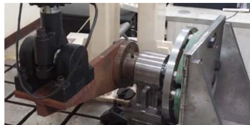
Figure 11: Disc pack torque transmission test
