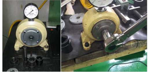
Figure 7: Torque coefficient test method
