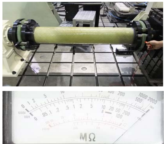
Figure 14: High speed coupling insulation resistance test and result
