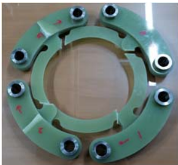
Figure 13: Fractured disc pack at 60kNm torque
