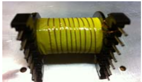
Figure 6: Sparse winding method (1~2mm)
