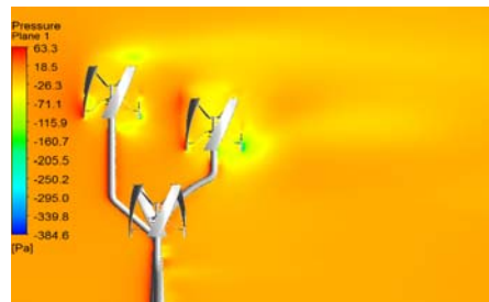
Figure 15: Pressure contour of the wind turbine tree under +Z wind direction
