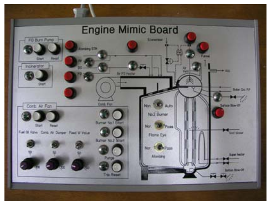
Figure 6: Auxiliary boiler mimic board
