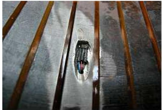
Figure 5: Hall effect sensor for measuring air-gap magnetic flux
