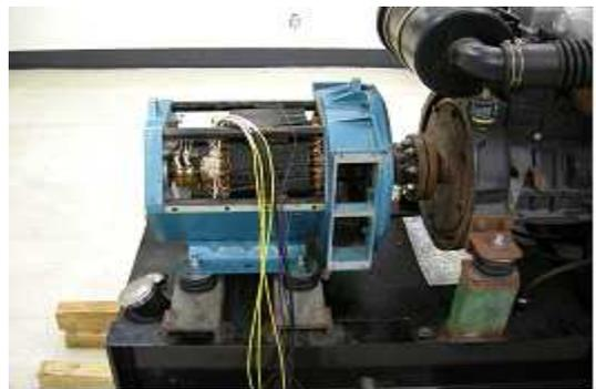
Figure 6: 2 pole synchronous generator for fault test
