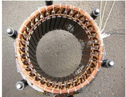
Figure 2: Stator for synchronous generator
