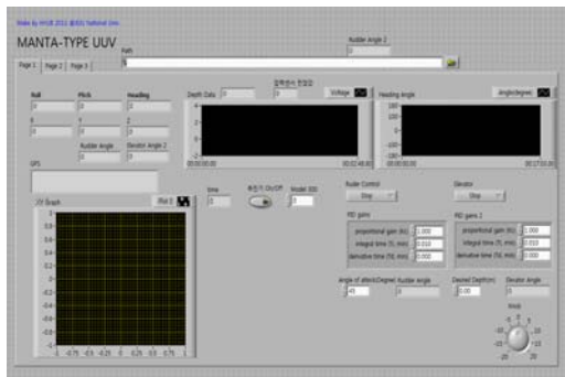
Figure 10: Control Program(Front Panel)
