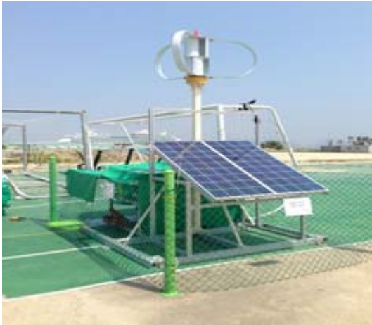
Figure 4: External appearance of hybrid power generation system
