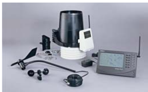
Figure 3: Parts of Weather Station [5]
