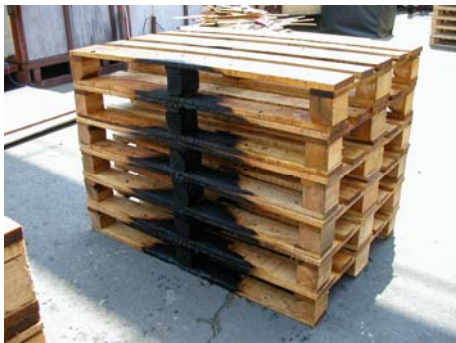
Figure 6: Damage to the fuel package
