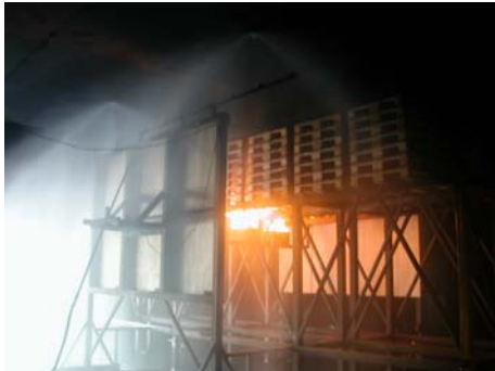
Figure 5: Water mist discharge
