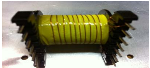
Figure 5: Low density windings (between gap 1~2 mm)
