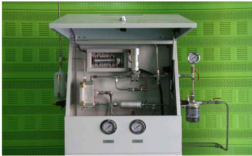
Figure 3: Test setup for Fuel Consumption Meter
