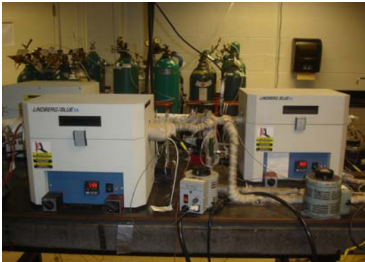
(c) View of steam generator and furnace for SCR
