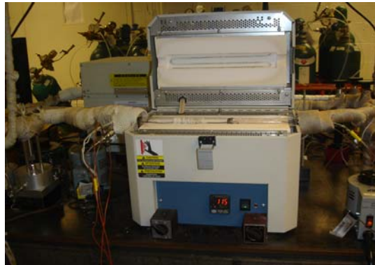
(d) Furnace with installed Cu-Chabazite sample
