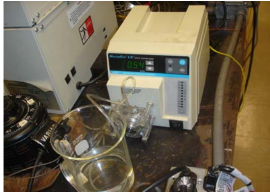
(b) Peristaltic pump of water injection for steaming
