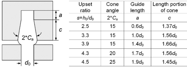
Figure 2: Schematic illustration of the preform geometry and design parameters
