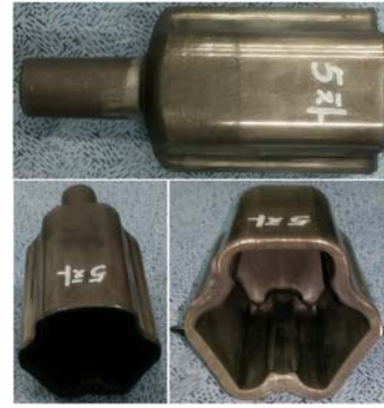
Figure 16: Hot forged tripod housing (5 th test operation)
