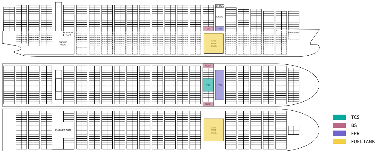
Figure 7: General arrangement of LNG fuelled containership
