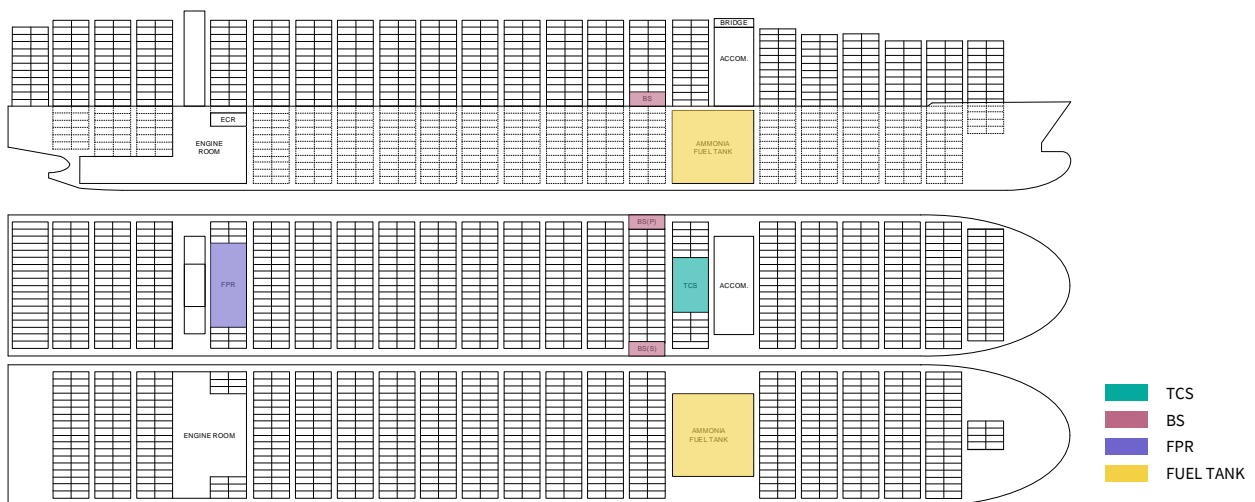
Figure 9: General arrangement of Ammonia fuelled containership
