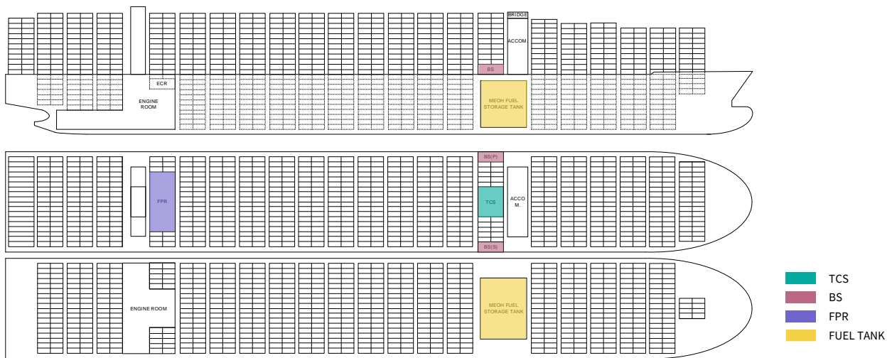
Figure 8: General arrangement of Methanol fuelled containership
