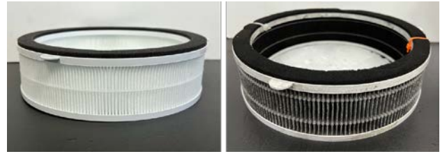
Figure 14: Photographs of Normal and Contaminated Filters Installed in Ships
