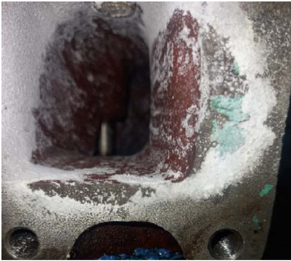
Figure 9: Photograph of the intake port with urea sedimentation
