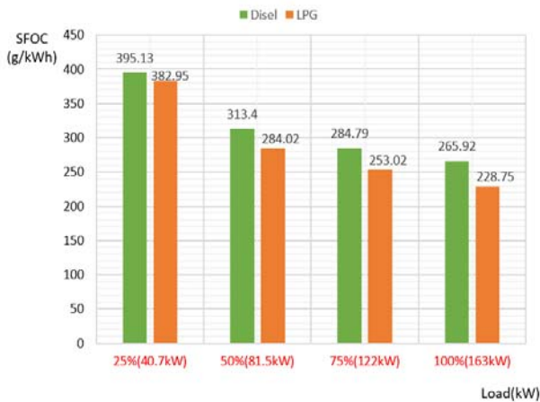
Figure 9: Comparison of diesel engine and LPG engine (SFOC)
