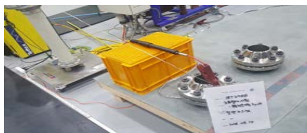
Figure 10: Partial discharge test and breakdown voltage test
