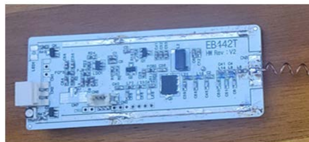
Figure 5: Electronic buoy transmitter device for monitoring fishing nets
