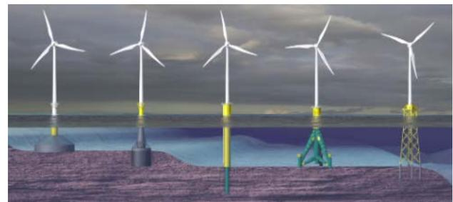
**Figure 1:** Fixed offshore wind turbine substructures
