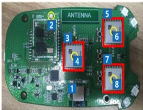
Figure 7: Multi-GPS seawater drifting device embedded board
