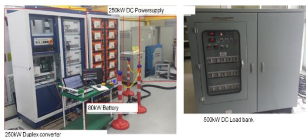
Figure 5: Test system for the hybrid RTGC
