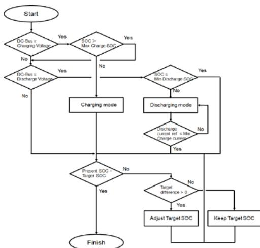
Figure 3: Control algorithm of the RTGC system
