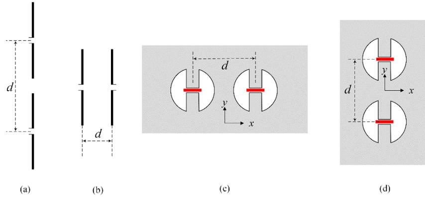
**Figure 4:** Array definitions according to arrangements of two dipole antennas and two RCAs. (a) Collinear and (b) side-by-side arrangements of the two dipoles. (c) Collinear and (d) side-by-side arrangements of the RCAs. The center-to-center distances of  $d$  are described for each case.
