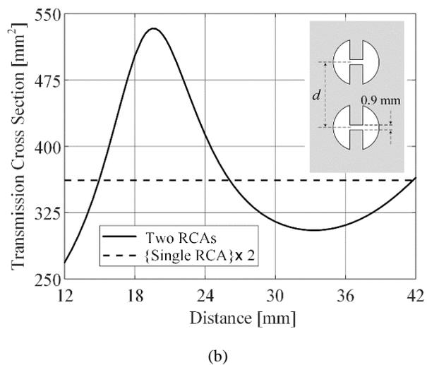
**Figure 5:** TCSs versus center-to-center distances for (a) collinear and (b) side-by-side arrangements in Case B2.
