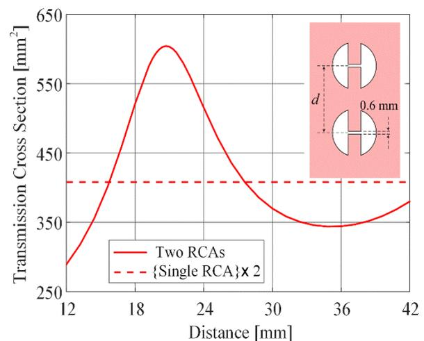
**Figure 7:** TCS versus the center-to-center distance for the collinear arrangement in Case B3.
