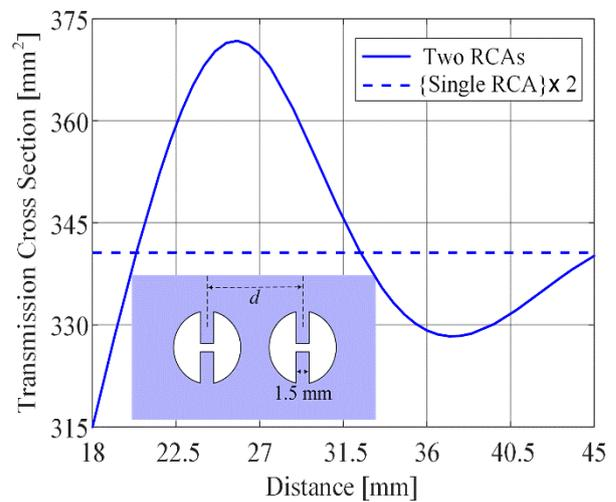
**Figure 6:** TCS versus the center-to-center distance for the collinear arrangement in Case A2.
