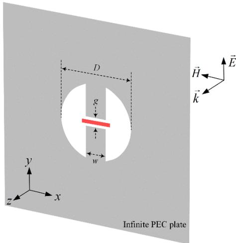
**Figure 1:** Single-ridged circular aperture perforated on a thin infinite perfect electric conductor screen. The aperture's variables are described, and the plane's electromagnetic wave is incident along the +z direction. The concentrated incident electric field is described in red along the x-axis and can be transformed into an equivalent magnetic current element.
