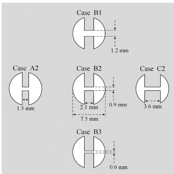
**Figure 2:** Five RCA cases are shown as functions of the ridge width  $w$  and gap  $g$  between the two ridges. The TCSs were tested for each RCA case.
