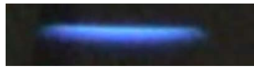
Figure 9: Image of counter-flow flame captured using a digital camera
