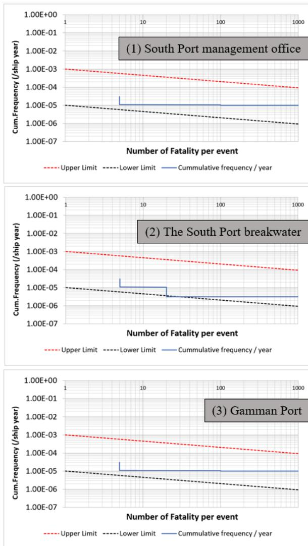
Figure 7: Results of PDA with F-N curves
