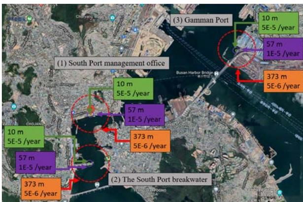
**Figure 6:** Proposed safety zones for three different bunkering locations
