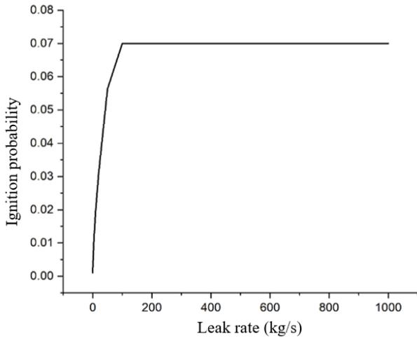
**Figure 3:** Ignition probability vs ammonia leak rate (kg/s)
