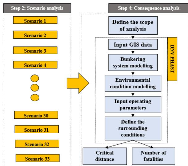
**Figure 4:** Process of consequence analysis
