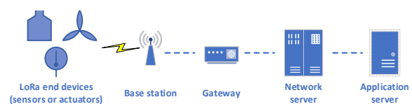
Figure 1: LoRaWAN network architecture
