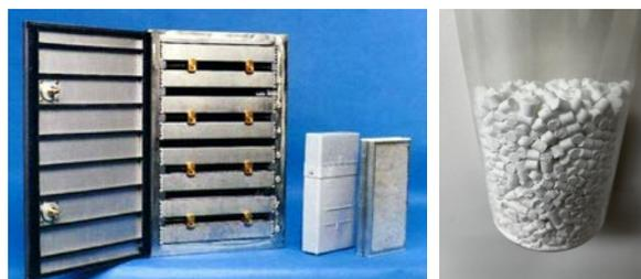
**Figure 2:** Scrubber and LiOH granules for the submarines
