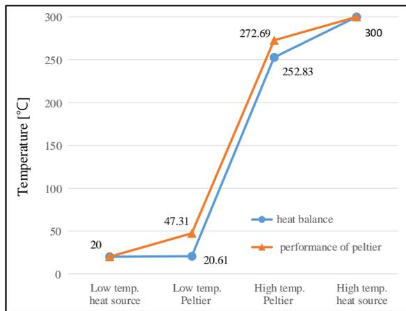
**Figure 3:** (CASE 1) Temperature profiles of the thermoelectric generator system
