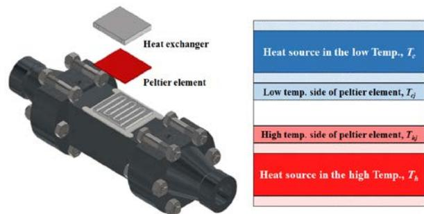
**Figure 1:** Thermal analysis model of the thermoelectric generator system
