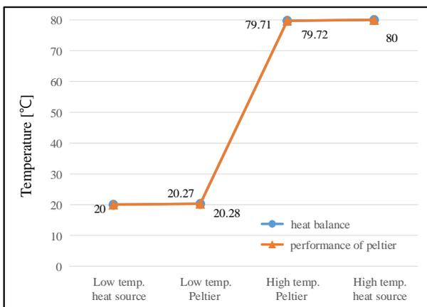
**Figure 6:** (CASE 4) Temperature profiles of the thermoelectric generator system
