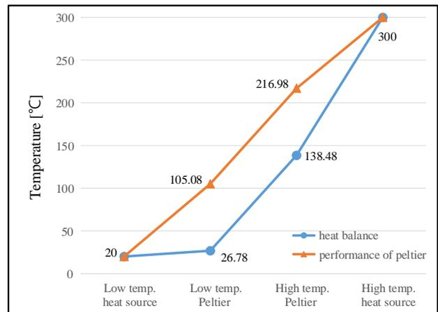
**Figure 5:** (CASE 3) Temperature profiles of the thermoelectric generator system
