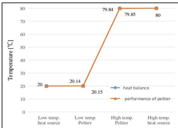
**Figure 4:** (CASE 2) Temperature profiles of the thermoelectric generator system
