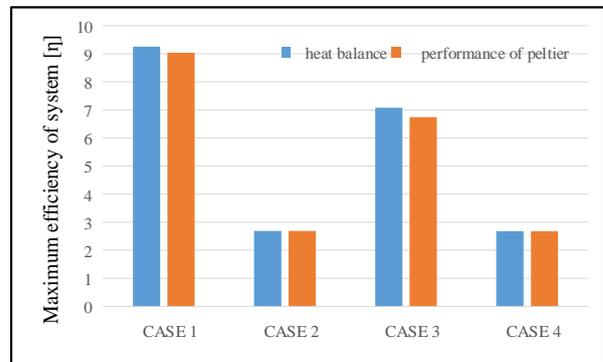
**Figure 7:** Maximum efficiency of the thermoelectric generator system
