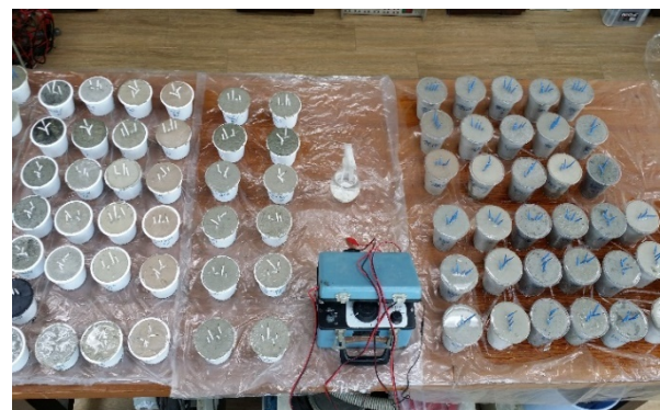
Figure 3: Resistivity measurement of mortar specimens
