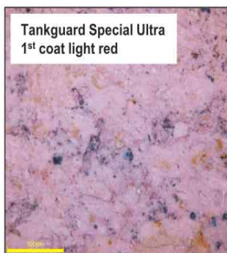
Figure 6: Contaminants of steel dust on the inner coating
