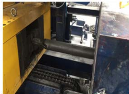
Figure 12: Drawing process of bilayered pipe
