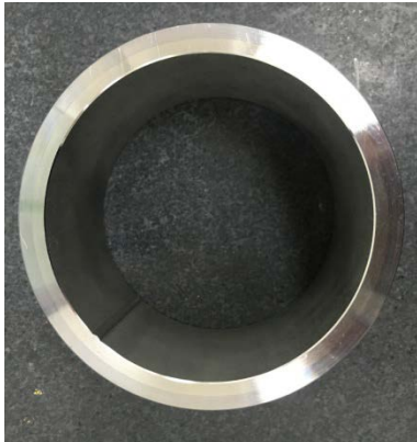
Figure 13: Indentation strength test of bilayered material pipe
