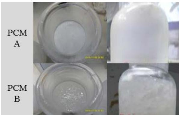
Figure 4: PCMs in beaker frozen by refrigerator
