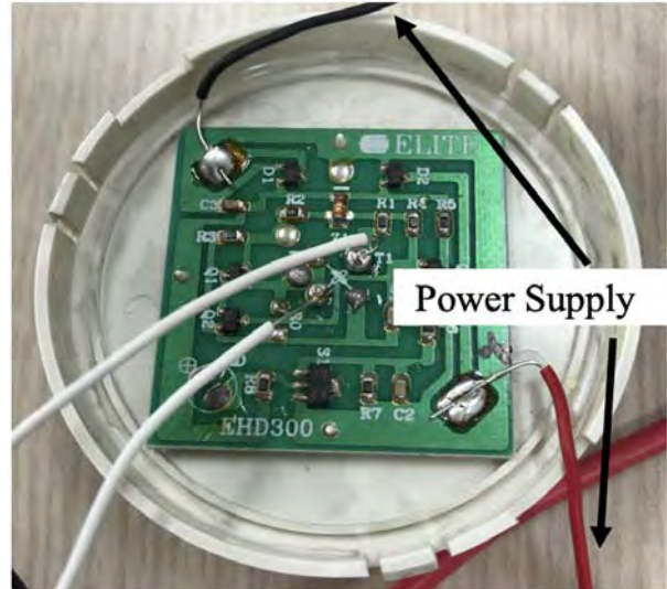
Figure 8: Connecting the BT signal detecting module and a power supply unit to the fire detecting sensor
