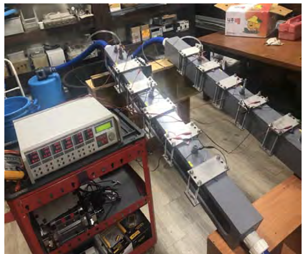
Figure 2: Overall appearance of test apparatus for cathodic protection in the piping experiment
