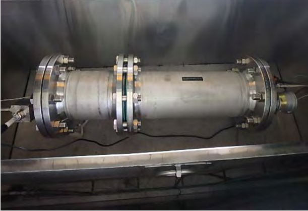
Figure 2: Installation of test sample for PTS
