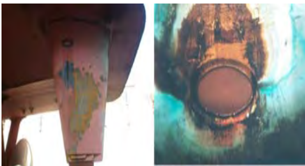
Figure 1: The case of corrosion rudder and ICCP of ○○ ship
