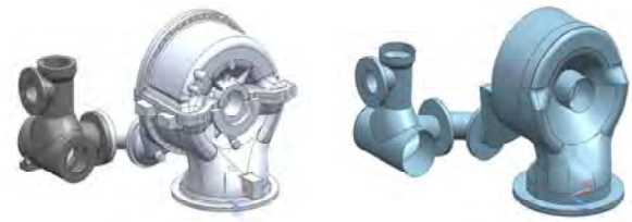
(a) 3D CAD model (b) Mid-surface model Figure 6: Geometric configuration for a casing of a steam turbine
