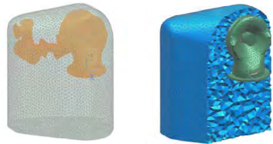
(a) Convex mesh (b) Fluid mesh Figure 8: Exterior fluid mesh model
