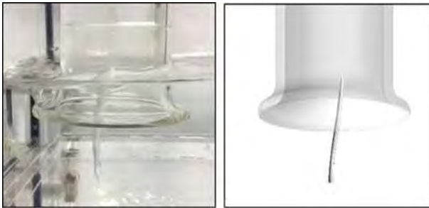
Figure 10: Comparison of numerical and experimental submerged vortex
