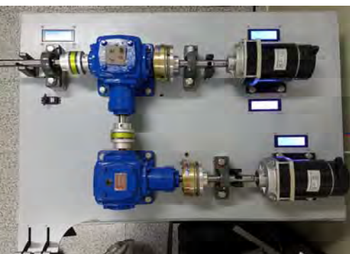
Figure 11: Propulsion system simulator layout
