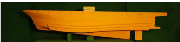
Figure 4: The model ship used to resistance tests of the appendages
