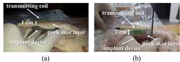
Figure 14: Wireless charging test in pork at distances of (a) 10 mm and (b) 20 mm
