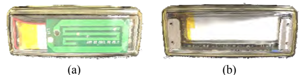
Figure 3: Developed ECG implant device prototype (a) front view and (b) rear view
