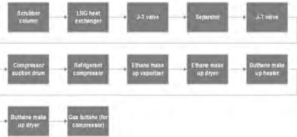
Figure 11: RBD of liquefaction & refrigeration modules
