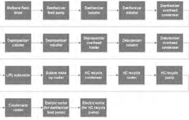
Figure 12: RBD of fractionation module
