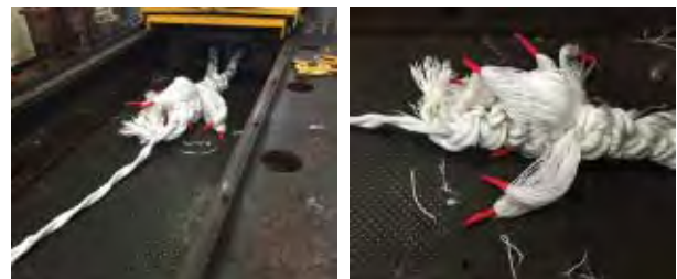
Figure 3: Tensile strength test of HDPE rope
