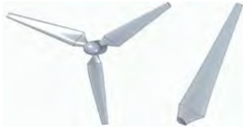
Figure 2: 3-D modelled 1MW HATT rotor blade
