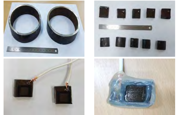
Figure 1: Carbon steel pipe specimen preparation for electrochemical polarization test
